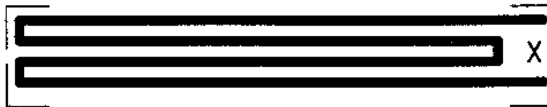
Figure 6-15: Example of test pattern for testing resistance to bending cycles
