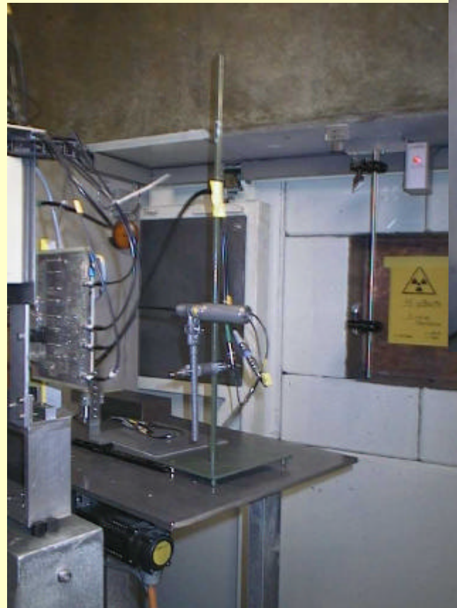
PKC2 XY-table, Laser and Beam Dump
