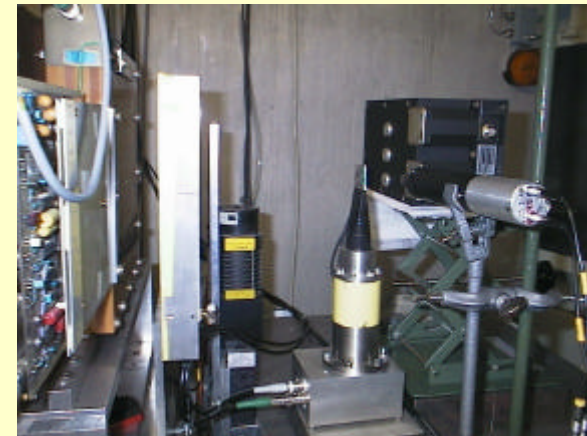
PROBA SREM mounted on PIF-PKC2 XY-table
