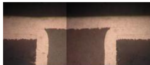
Figure 9. Cross-section of cap plating
