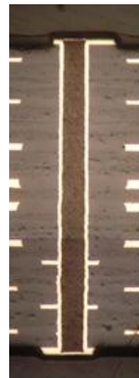
Figure 8. Cross section of 0.2mm Dia. PTH
