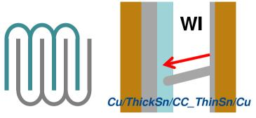
Type 2: Monitors whisker penetration in through coating
