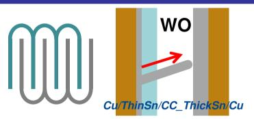
Type 1: Monitors whisker penetration out from under coating
