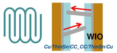
Type 3: Monitors whisker penetration out from under coating and in thorough coating
