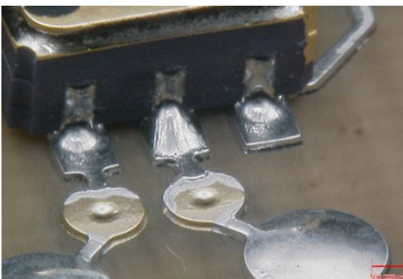
Figure 5. LCC6 after vapour phase soldering assembly
