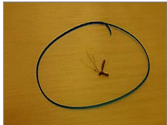
Fig. 9. Top view of a prepreg showing an embedded insect.
