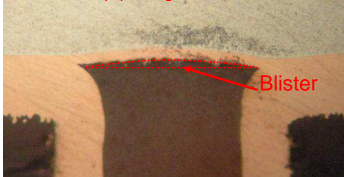
\phi 0.2mm Cap plating thickness 0.020mm
