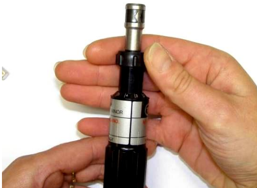
Set up the torque level to: 0.08Nm (0.71 inch-pounds) torque for electrical test purposes 0.10 Nm (0.89 inch-pounds) min to 0.12 Nm (1.06 inch-pounds) max torque for mechanical test or flight purposes*
