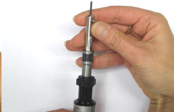
Insert the 0.050" bit for Hex screw into the screwdriver
