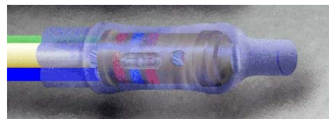
Figure 19-24. Contact Covered With Shrink Sleeving
