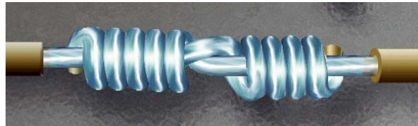
Figure 19-16. Completed Wrap for Western Union/Lineman Splice
