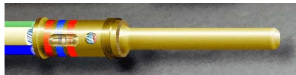
Figure 19-22. Wires Crimped Within Contact
