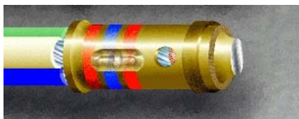
Figure 19-23. Contact Trimmed and Deburred
