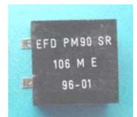
Fig. 34: Verification of the measurements with a stable capacitor PM90SR
