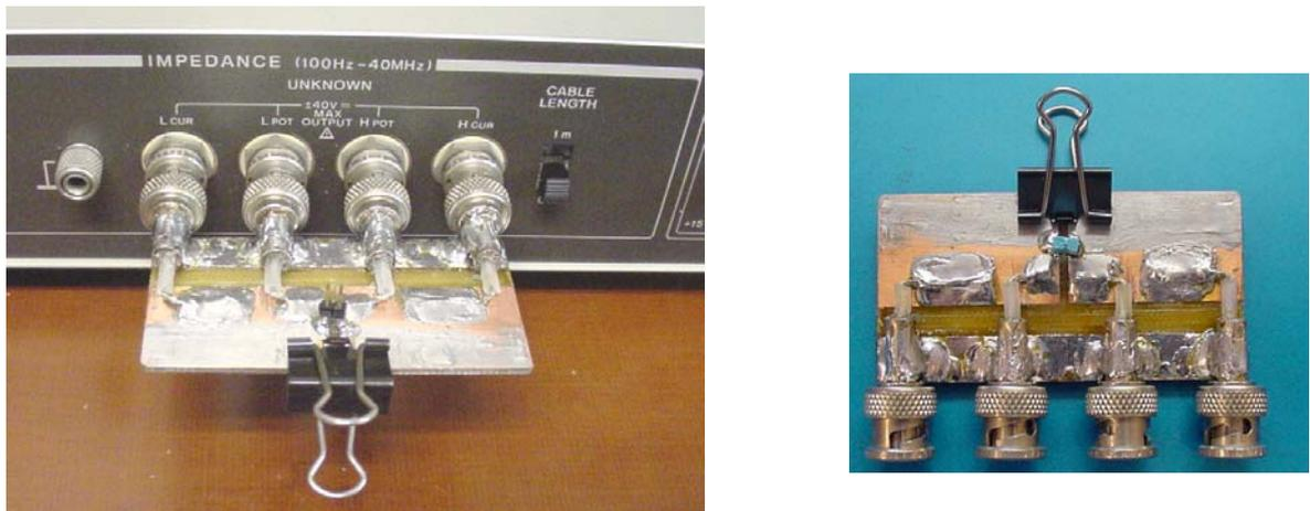
Fig. 41a and b: Frequency Analyser and its clip connector
