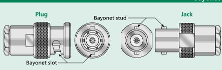
Bayonet mating is used where a quick mating and unmating action is desired, and accidental disconnection by pulling on the cable must be prevented.
