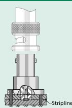
Used to transmit signal from a strip transmission line.
