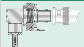
Used to transmit signal from a cable through a panel, using a single mounting hole.
