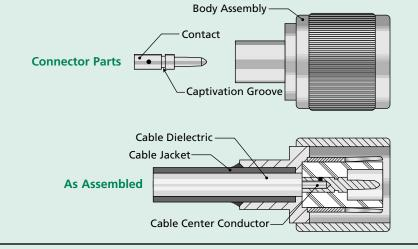
Direct-solder attachment is the most efficient method of attaching semi-rigid cable.
