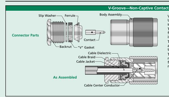
V-Groove cable attachment is the standard for military UG-type connectors, and is field-replaceable with no special tools.
