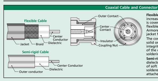
Flexible cable: Center conductor (solid wire, or stranded wire for increased flexibility) is contained within a tubular dielectric, which is covered by braided shield wires and a protective jacket. Many flexible cables have a second layer of braid for increased shielding. Armored cables have a layer of braided flat steel wires over the jacket for abrasion resistance.
