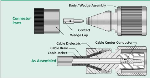
This unique attachment system provides very fast assembly and is field replaceable.
