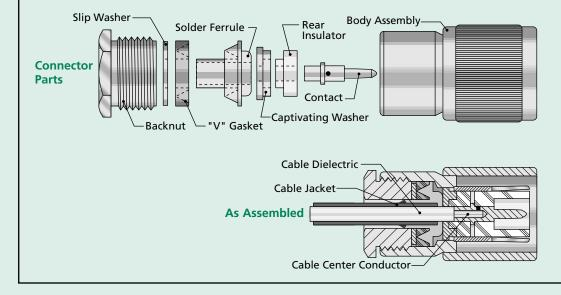
This attachment method is similar to the V-Groove type used for flexible cable, but is adapted to use with semi-rigid cable by replacing the braid-clamp ferrule with a ferrule designed to be soldered to the jacket (outer conductor) of semi-rigid cable.
