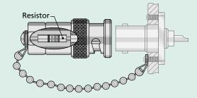
Used to simulate a load in an incomplete circuit.
