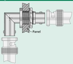
Used to transmit signal through a panel, using a single mounting hole, and connect two plugs.
