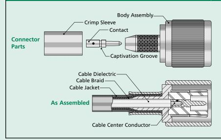
These connectors offer quick assembly time and small size, and feature a captive contact which snaps into place in the insulator when assembled. This provides consistent axial contact location within the interface, and prevents movement of the contact from cable flexure or temperature changes after assembly.
