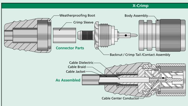
X-Crimp cable attachment combines ease of assembly with a captivated contact and a silicone-rubber boot\* for weatherproofing.
