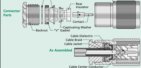
V-Groove clamping with a captive contact provides consistent axial contact location within the interface, and prevents movement of the contact from cable flexure or temperature changes after assembly.
