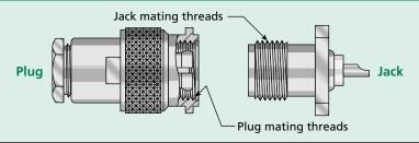
Threaded mating is used where secure mated condition is desired (or where connector interface characteristics require a specific amount of force), and space is available to turn the coupling nut.
