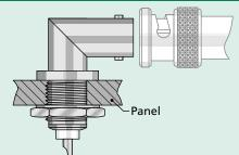
Used to transmit a signal from internal circuitry through a panel, using a single mounting hole. Best suited for use with thick panels.
