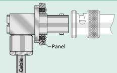
Used to transmit signal from a cable through a panel, using a flange with two to four holes to accommodate mounting screws or bolts. Best suited for use with thin panels.
