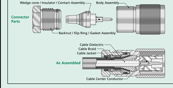
This patented attachment system features a captive contact, quick assembly, and secure cable retention. The cable braid and jacket are flared over the coneshaped wedge, and the backnut captures the braid and jacket when screwed into the body assembly.
