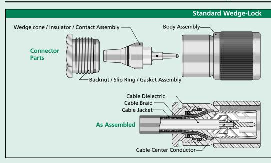
This patented attachment system features a captive contact, quick assembly, and secure cable retention.
