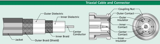
Similar to coaxial construction, but with an additional layer of dielectric and braid shield.
