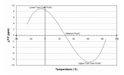
Figure 12: Typical frequency-temperature curve (AT-cut)
