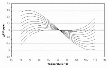
Figure 14: Frequency-Temperature characteristics of SC-cut for different values of θ
