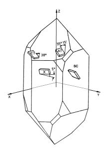
Figure 1: Orientation of different cuts in a natural quartz crystal
