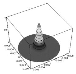
Figure 5: amplitude of vibration in the plate plan in a plano-convex resonator
