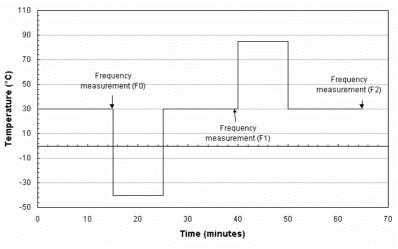
Figure 18: Temperature cycle
