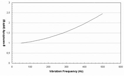
G-sensitivity is the frequency dependancy on the acceleration of the device.
