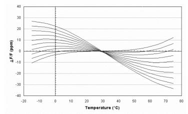
The frequency-temperature characteristic is primaraly determined by the the cut angle. For a given cut the parameter which changes the most with  $\theta$  angle is A<sub>i</sub>.
