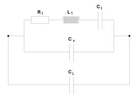
Figure 11: Load capacitance in parallel
