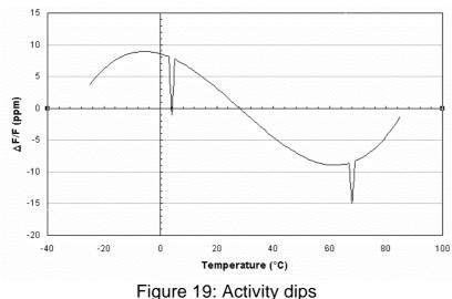
Dips can cause problems in crystals for VCXOs and TCXOs. A dip is characterized by deviation from the third order frequency-temperature curve.
