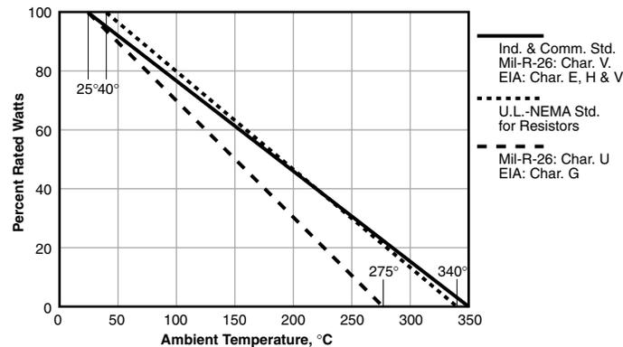
Fig. 4: Derating of Resistors for High Ambient Temperatures.
