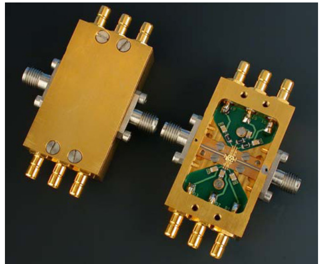
Fig. 8 : Line-up of a driver and power amplifier module.
