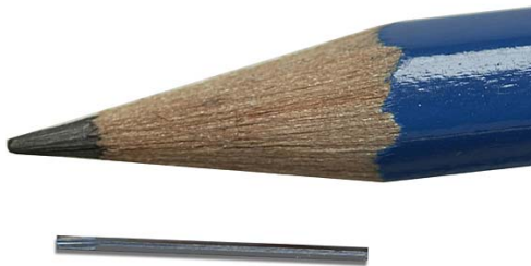
The MEMS sensing element compared to a pencil tip
