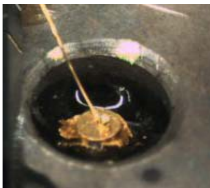
Compromised glass to metal seal
