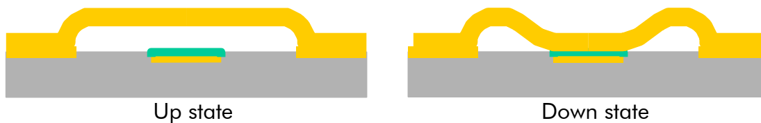
Figure 1 : Schematic cross section of a shunt MEMS switch
