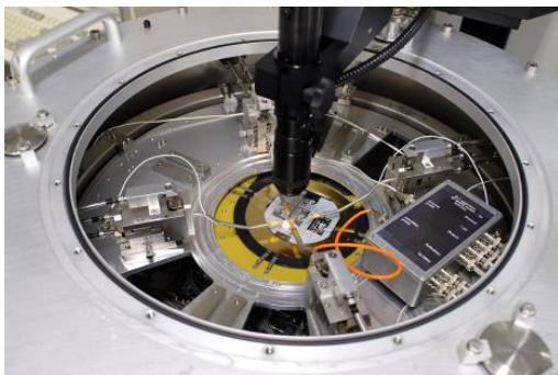
Figure 3 Fully automated ELT, C-V and stepping procedures within a controlled atmosphere chamber (PAV150, Suss MicroTec)
