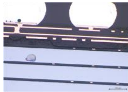
Figure 9: Internal failure after preconditioning and TC
