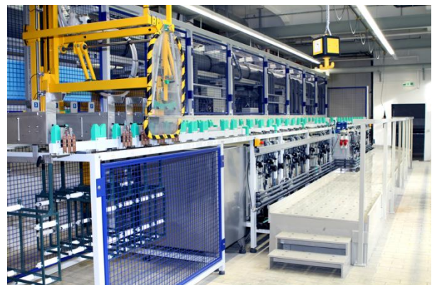
Figure 2. The ENIPIG-plating line (Galvabau) at Tesat Spacecom GmbH & Co.KG
