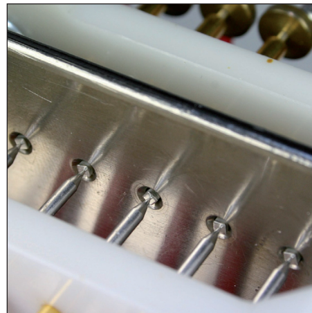
Fig. 11: Burn-in equipment with fuses
