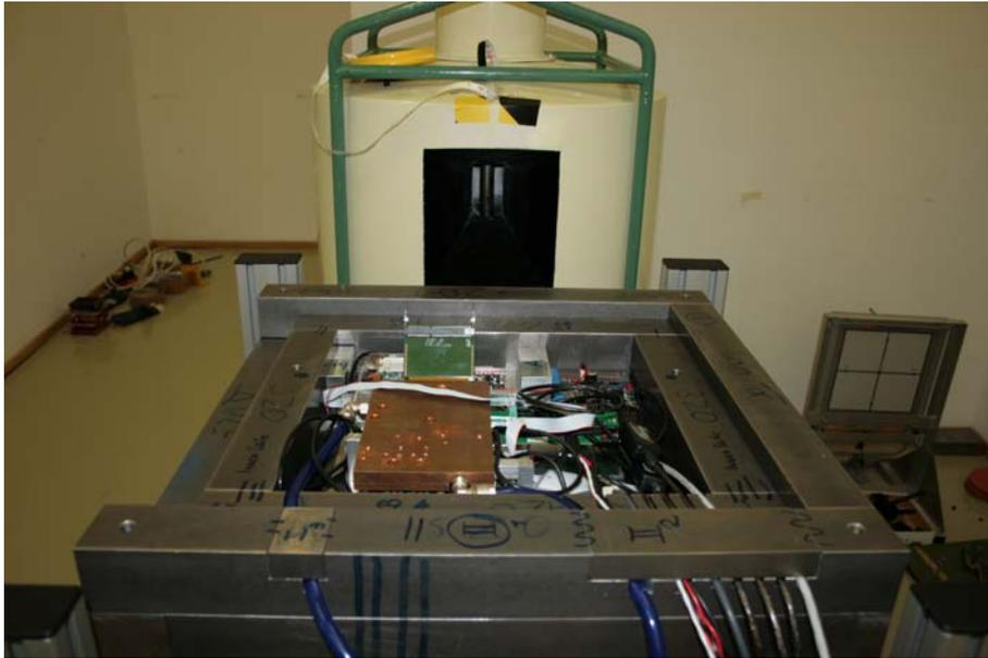
Figure 4: our test device in the shielding box, with the top part of the shielding box removed
