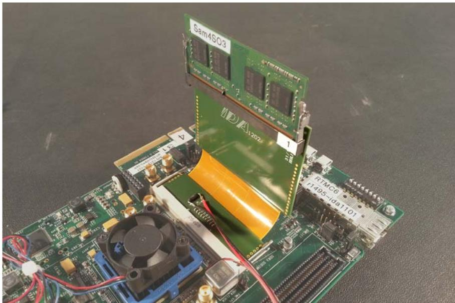
Figure 5: the flexible extension with an SODIMM in the ML605 (with a fan on the FPGA instead of the water cooler)
