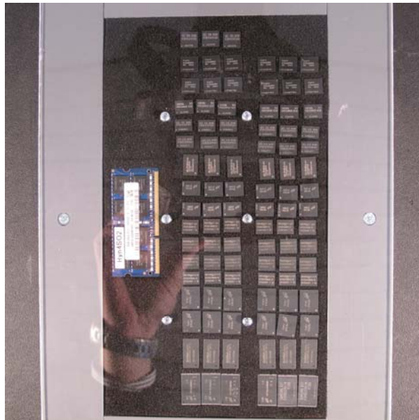
Figure 1: the DUTs in the plastic frame with an acrylic glass cover (without the aluminium foil)
