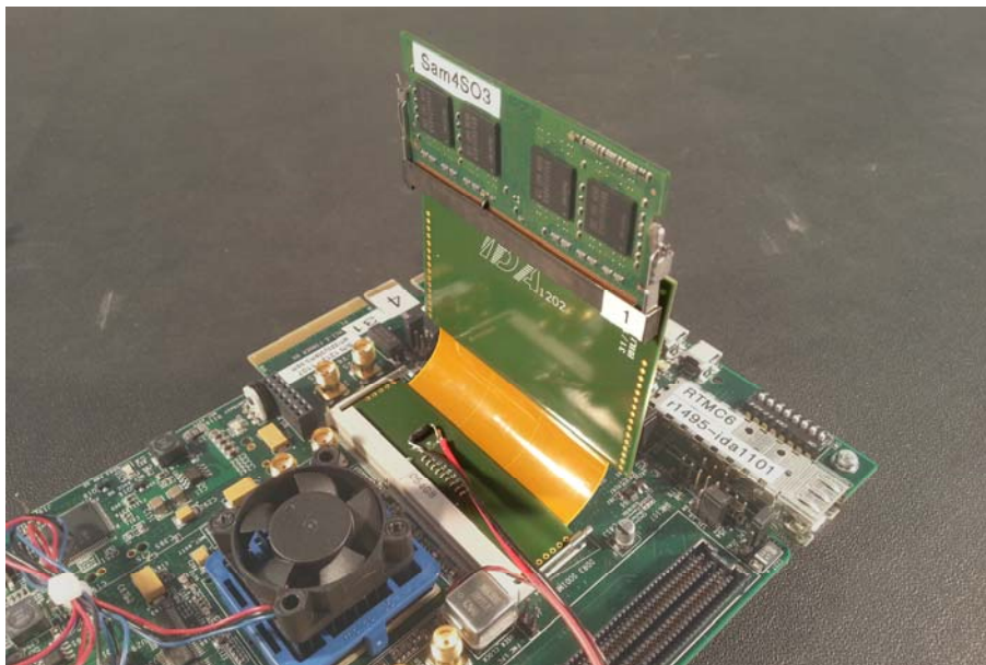
Figure 7: the flexible extension with an SODIMM in the ML605 (with a fan on the FPGA instead of the water cooler)
