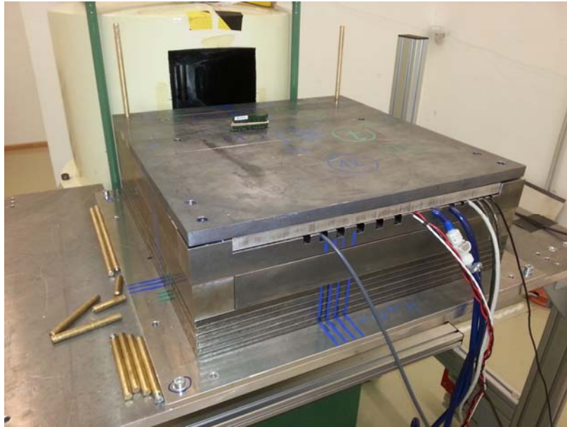
Figure 4: the shielding box with water tubes (blue) and electrical wires
