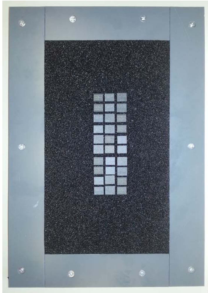
Figure 1: the DUTs in the plastic frame (without the acrylic glass and aluminium sheets)
