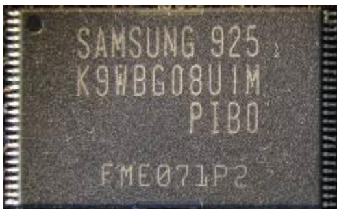
Fig. 18: Samsung K9WBG08U1M-PIB0 NAND-Flash
