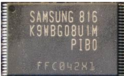
Fig. 17: Samsung K9WBG08U1M-PIB0 NAND-Flash
