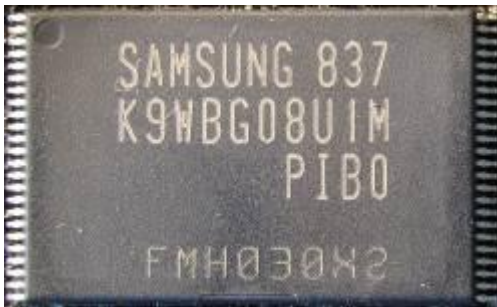
Fig. 16: Samsung K9WBG08U1M-PIB0 NAND-Flash
