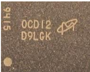
Fig. 14: Micron MT41J256M8HX-15E:D DDR3 SDRAM
