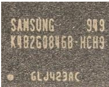
Fig. 13: Samsung K4B2G0846B-HCH9 DDR3 SDRAM
