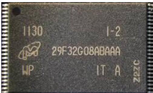
Fig. 41: Micron MT29F32G08ABAAAWP-IT:A NAND-Flash
