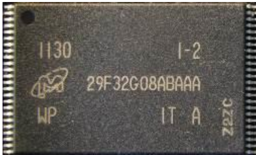
Fig. 21: Micron MT29F32G08ABAAAWP-IT:A NAND-Flash
