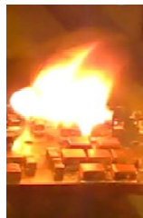
Fig. 4. Snapshot of a “Transient Thermal Event” in a Failing MnO 2 -Cathode Tantalum Capacitor.
