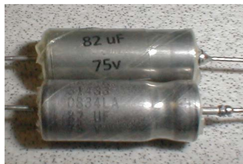
Fig. 4. Hermetically sealed Polymer (top) and Wet (bottom) Ta capacitors B-cse 82 \mu\text{F} – 75 V.
