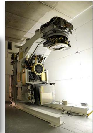
**2. New ion Beam Combination.** Complete the construction of the new HIISI (Heavy Ion Ion Source Injector) 18 GHz ECR ion source so, that K-130 accelerator is able to produce more energetic ion beam combination, aiming 15 MeV/u in energy. The new cocktail would include also heavier ion than Xe, e.g. Au.
