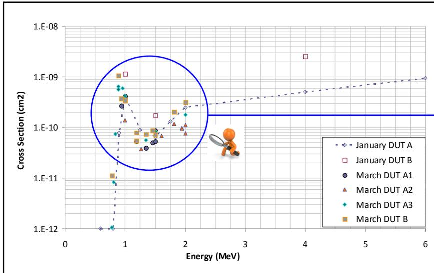
Proton cross section  $\sigma(E)$  between 0.75 and 2.25 MeV
