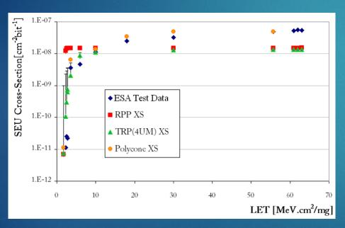
Reconstruction of Proton SEU crosssection test data for the RSEUM
