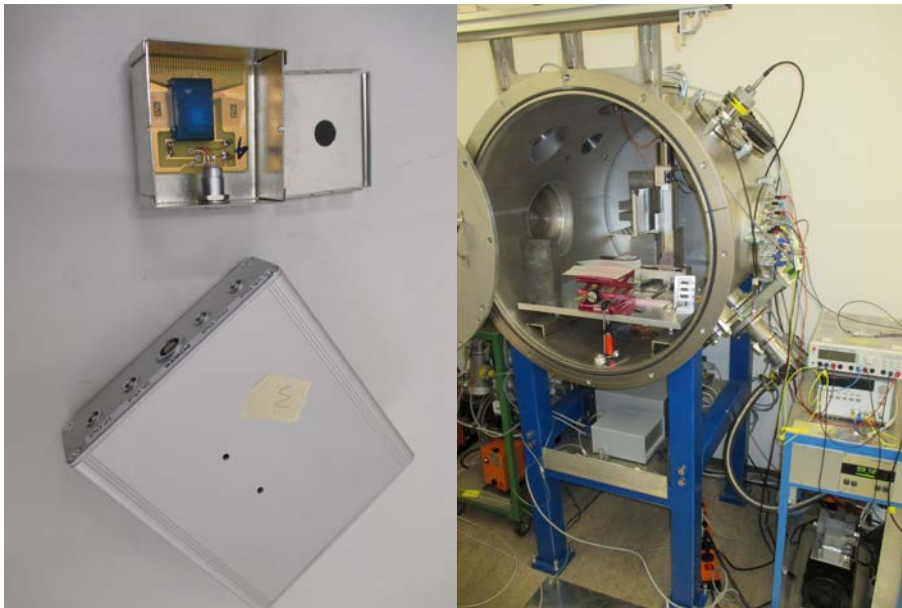
Si-detector and DAQ system (left); Monochromator chamber (right)
