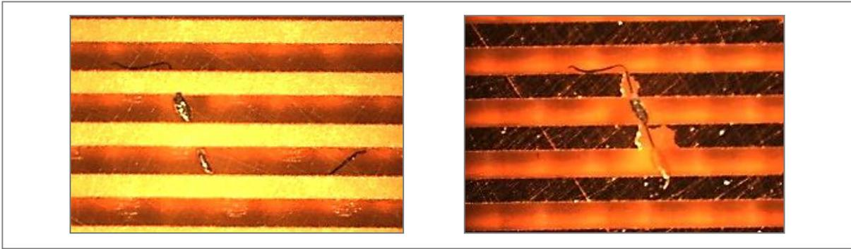
Fig. 7. In-plane sections of comb pattern after progressive polishing showing copper migration from the conductor along the fiber contamination.
