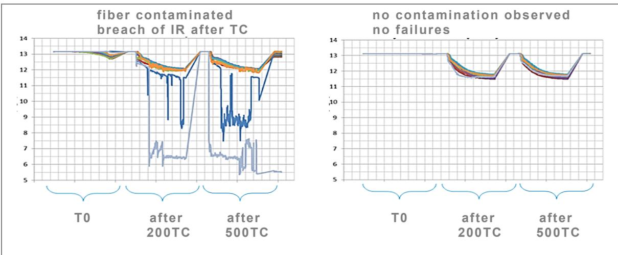
Fig. 6. Insulation resistance ( $\log \Omega$ ) before and after thermal cycles (TC) from  $-65^{\circ}\text{C}$  to  $+135^{\circ}\text{C}$ , showing two failed innerlayers of a comb pattern that appeared to be fiber contaminated.
