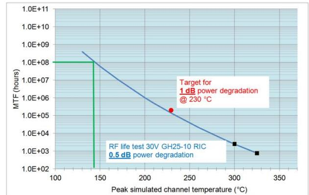
Figure 15: GH25-10 GaN-MMIC life time extrapolation for wear-out failure mode (failure criterion: 0.5 dB RF output power degradation)
