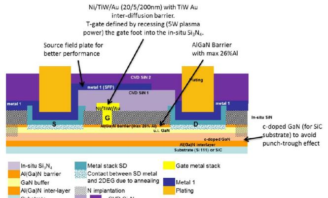
Figure 4: Schematic cross-section of the latest imec GaN RF device generation developed within GREAT<sup>2</sup>
