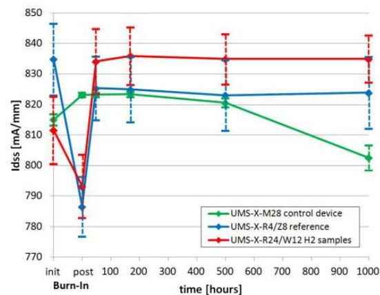
Figure 17: GH25-10  $I_{dss}$  evolution during 1000 hours hydrogen test (mean value of 12 samples +/- the standard deviation as error bar shown)
