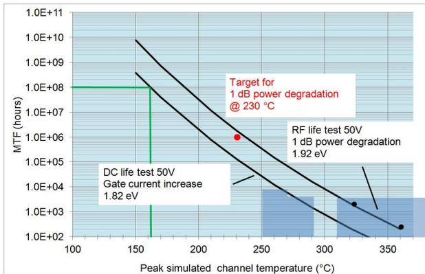
Figure 12: GH50-10 power cell life time extrapolation for wear-out failure mode (failure criterion: 1 dB RF output power degradation from RF life test and UMS DC life test data)
