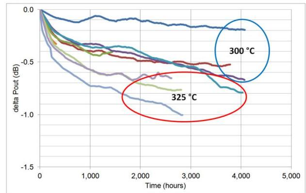
Figure 14: GH25-10 MMIC output power degradation at 300 °C and 325 °C channel temperatures
