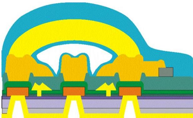
Figure 6: Schematic cross section of the active region of a GH50-10 transistor
