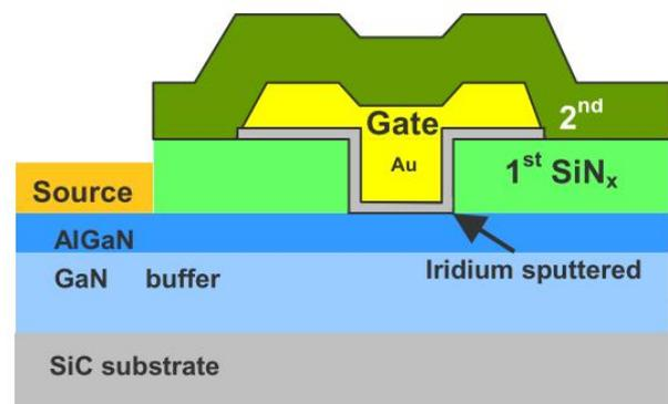
Figure 1: Sketch of FBH gate module with sputtered Schottky gate
