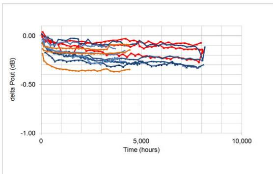
Figure 13: GH50-10 power cell output power degradation at 250 °C to 290 °C channel temperatures RF life test
