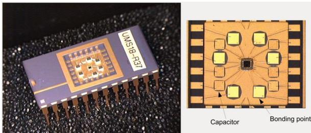
Figure 8: Radiation PCM assembled in DIL24 package
