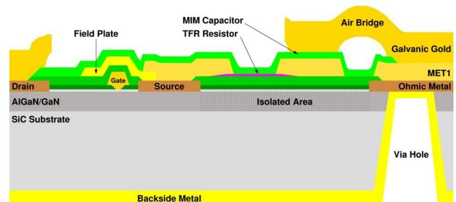
Figure 7: GH25-10 process schematic cross section
