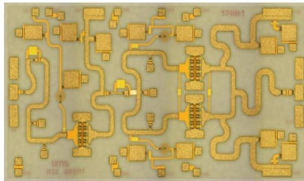
Figure 10: UMS GH25 GaN X-Band MMIC ( $4.1 \times 2.2 \text{ mm}^2$ )
