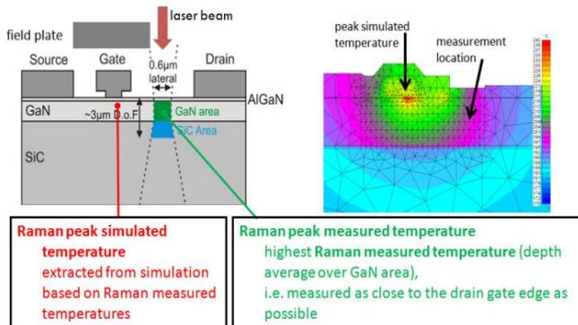
Figure 5: Raman thermography and temperature definitions used for GREAT<sup>2</sup>
