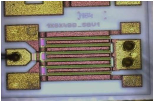
Figure 9: UMS GH50-10  $6 \times 400 \mu\text{m}$  power cell
