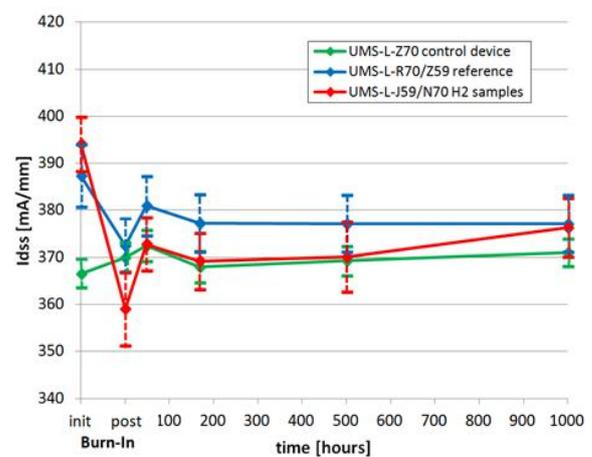
Figure 16: GH50-10  $I_{dss}$  evolution during 1000 hours hydrogen test (mean value of 12 devices +/- the standard deviation as error bar shown)
