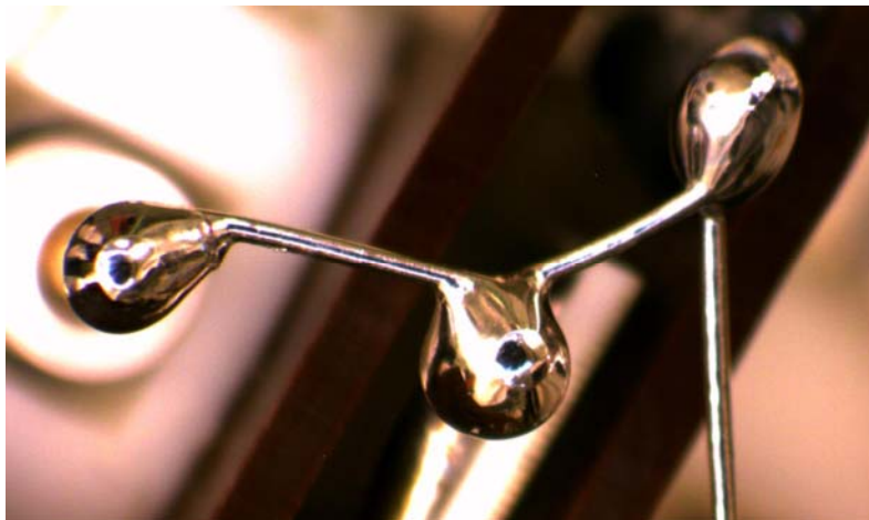
Figure 5-5: Examples for practical: connections of wires by using spherical solder joints
