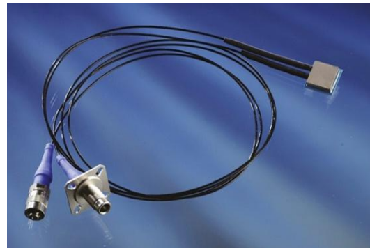
Engineering Model of (6.25 Gbps) SpaceFibre transceiver
