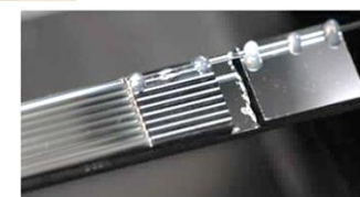
Optical interconnects on printed circuit board, and polymer waveguides
