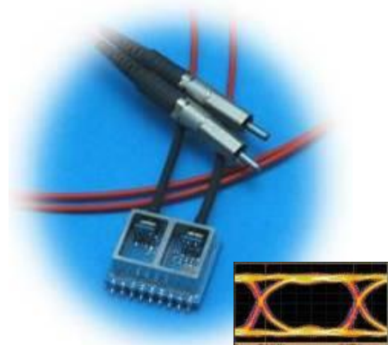
1 st gen (3 Gbps) SpaceFibre prototype
