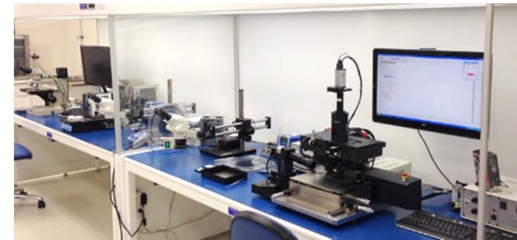
Finetech Fineplacer (0.5 micron accuracy)
