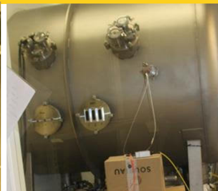
Low temperature test set 10-9 Bar liquid nitrogen
