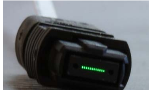
High density connector selected: 12 optical fibers MPO type
