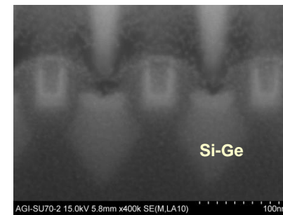
28nm CMOS Si-Ge transistor
