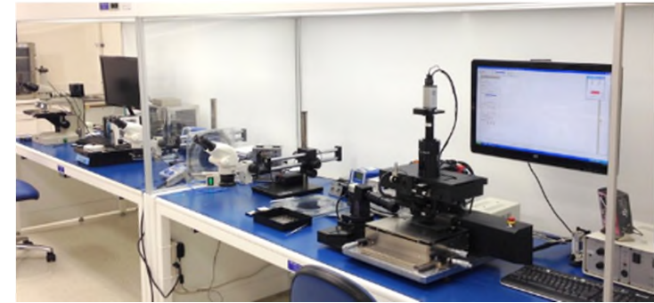
Finetech Fineplacer (0.5 micron accuracy)
