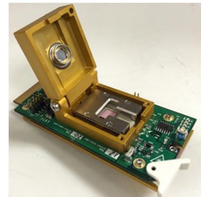
Transceiver Test Station with unique Optical Power Monitoring During Burn-In
