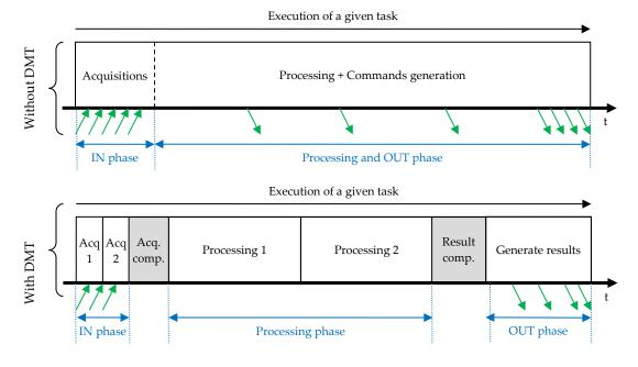
Figure 14-8: Scheduling and fault detection in DMT architecture
