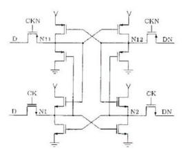
Figure 9-7: NASA-Whitaker hardened memory cell
