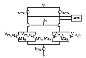
Figure 8-21: Simplified circuit schematic of the differential amplifier showing the split input paths (From [142])
