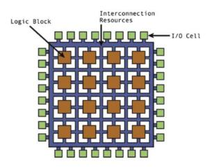
Figure 13-1: High-level description of an FPGA structure
