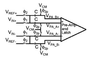
Figure 8-22: The switched-capacitor comparator with split differential amplifier input paths to harden the floating nodes against single-event upsets (From [142])
