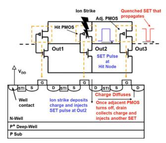
Figure 8-16: Two-dimensional slice of three PMOS transistors depicting the electrical signal and the charge-sharing signal caused by an ion strike, i.e. pulse quenching (From [142]).
