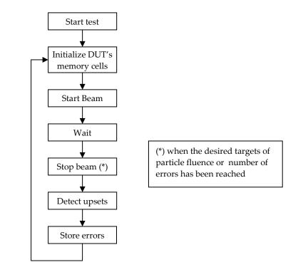
Figure 16-2: Flow chart of a typical static test
