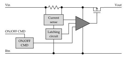
Figure 15-5: Block diagram of a LCL
