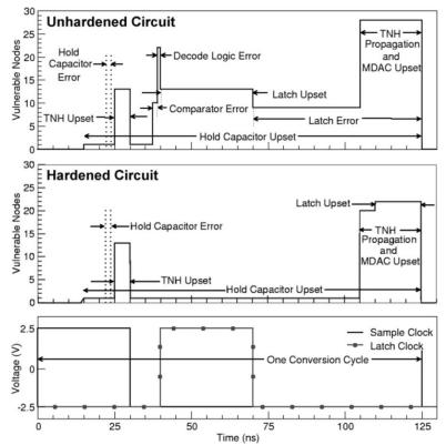
Figure 8-12: Simulated windows of vulnerability over one data conversion cycle for un-hardened and hardened 2-bit flash ADCs (From [132])
