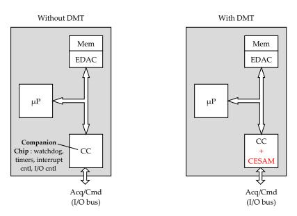
Figure 14-7: DMT architecture
