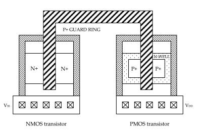
Figure 7-5: CMOS transistors with guard rings
