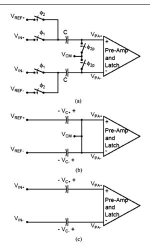
Figure 8-20: (a) The switched-capacitor comparator operates in two phases: (b) reset phase and (c) evaluation phase (From [142])
