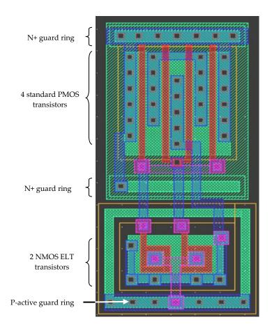
Figure 10-1: Hardened 2 input NOR gate
