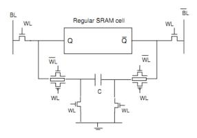
Figure 9-3: The SRAM-tct cell
