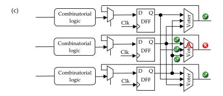
Figure 11-6: Fault detection and correction in the full TMR architecture
