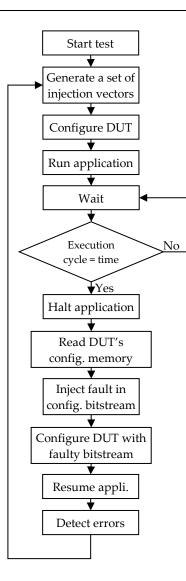
**Figure 16-1: Flow chart for fault injections in FPGAs**
