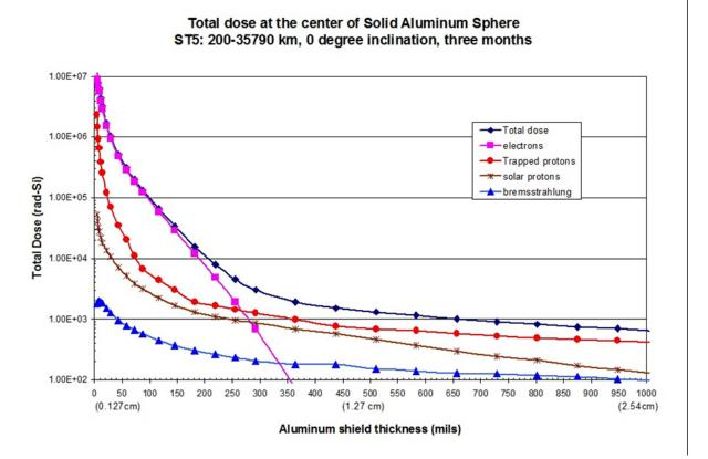
Figure 15-3: Example of a dose depth curve (C. Poivey, NSREC 2002 short course)
