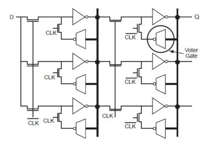
Figure 13-4: RTAX-S/SL/DSP R-cell Implementation of D Flip-Flop Using Voter Gate Logic
