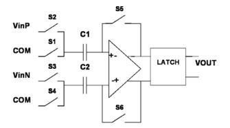
Figure 8-13: Simplified view of the auto-zeroed comparator (From [134])
