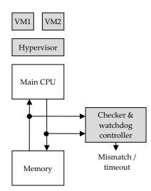
Figure 14-9: Time redundancy at application level
