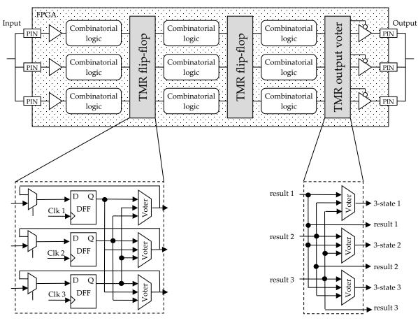
Figure 13-5: Global TMR implemented in an FPGA
