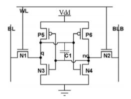
Figure 9-2: Hardened SRAM cell using a capacitor (SRAM-C cell)
