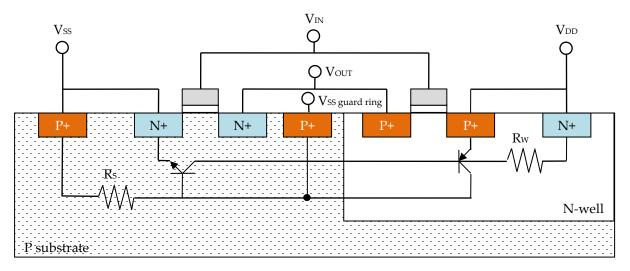
Figure 7-4: Parasitic thyristor responsible for SEL (top), introduction of P+ guard ring around NMOS transistor (bottom)
