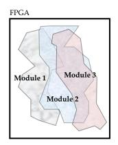
Figure 13-6: Physical implementation of global TMR inside an FPGA
