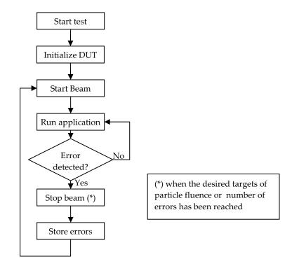
Figure 16-3: Flow chart for a typical dynamic test
