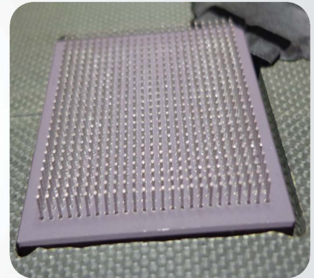
625 Columns on Ceramic package with a pitch of 1mm
