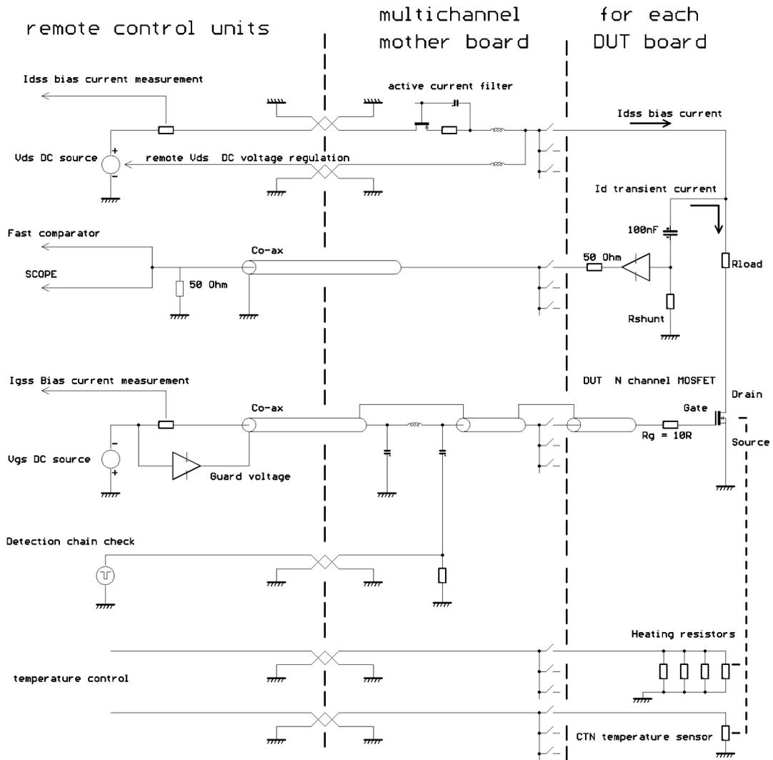
Figure 3 – Functional diagram for SEE Test
