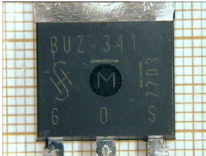
**Figure 1 – Device marking**
