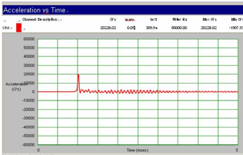
Figure 15. Shock test 20,000g, half-sine, 0.1ms
