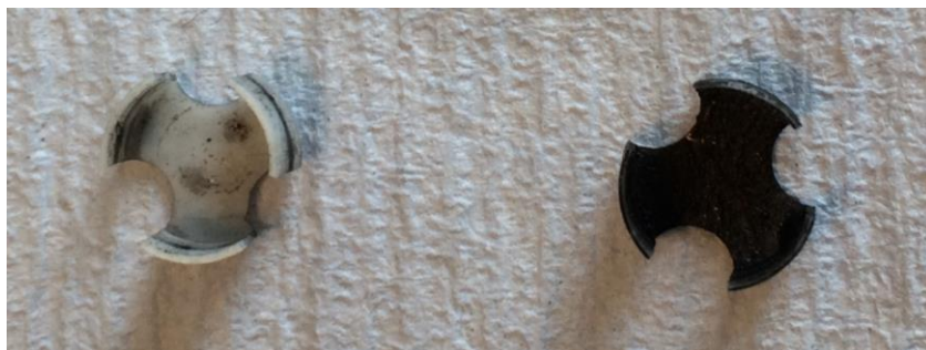
Fig. 4. Buildup of tantalum pentoxide following wet tantalum capacitor vibration testing
