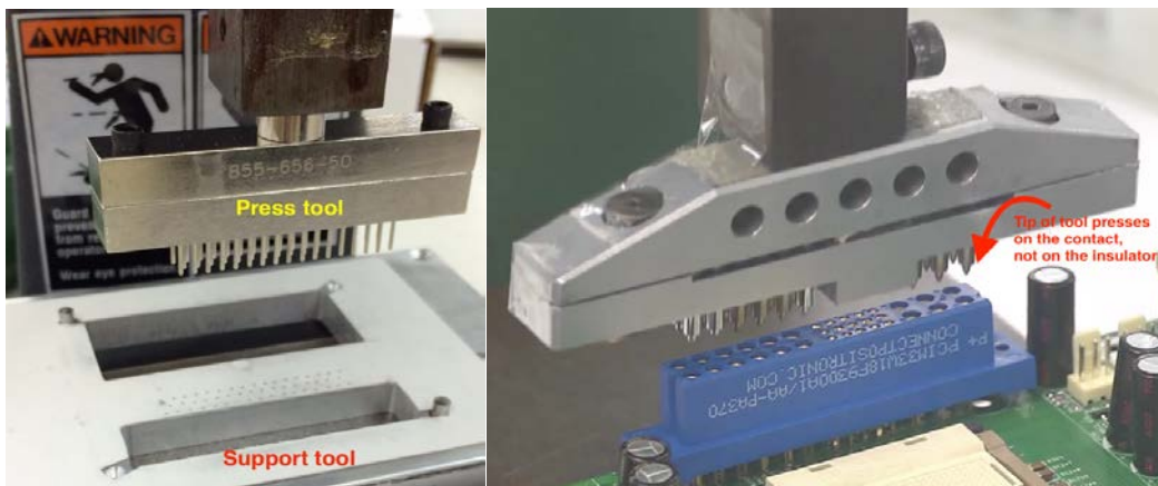
Fig.4b: Press tools and their action
