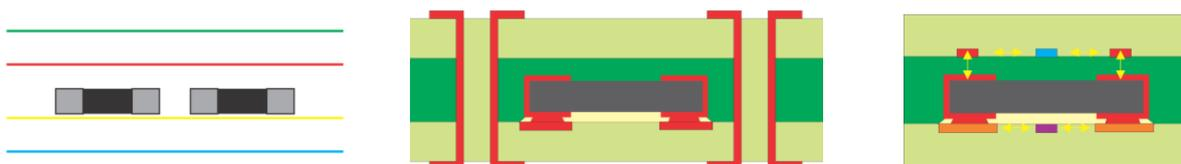
Fig. 3. Test structures for board-level insulation: disc (left), tree (middle) and comb (right)
