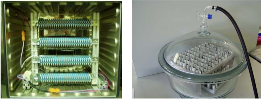
Fig. 18. EGGO supercapacitors screening facilities - burn-in (left) and vacuum (right)
