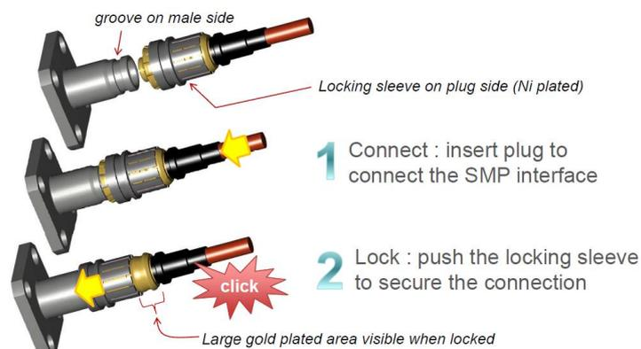
Fig1 : Mating sequence of SMP-LOCK connectors
